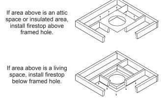
Figure 20 - Installing Firestop
